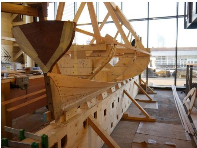
Our joinery module equips students with the hand tool skills required for boatbuilding. Students then move to boat work on the main floor, using both hand and static power tools. The College curates a wide variety of real, operational new builds and selected restoration projects of different sizes ready for student training tasks. This ensures that students gain experience of each stage, on craft from different era, constructed using a variety of techniques.
